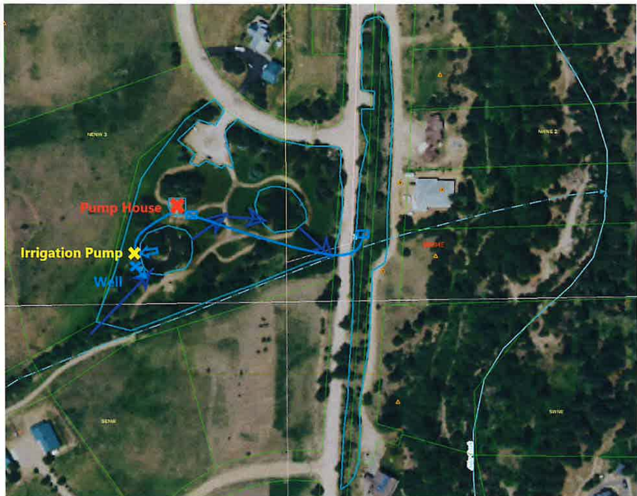
Figure 3- System diagram- Dark blue line (flow of water through ponds and ditches), Medium blue line (water lines from well and irrigation pump to control valves, Light blue outline (POU area).
