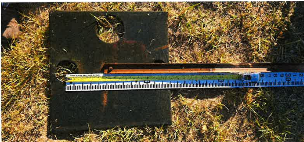
Figure 2: Measuring 3" Orifice (plate rotates to allow use of 1 of 3 orifices, 1.5", 3" & 4" diameter, allowing variable control of flow into the bypass pipe). The 4" orifice was used for the licensing measurement
