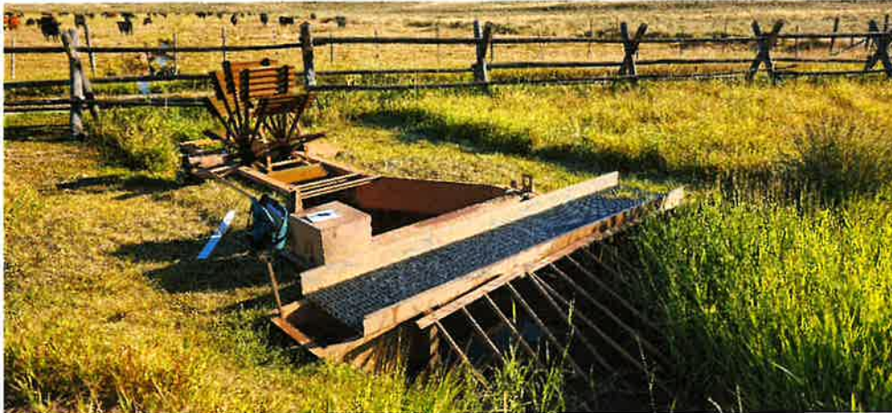
Figure 1: Fish screen with bypass (T-handle front left side located over bypass opening)
