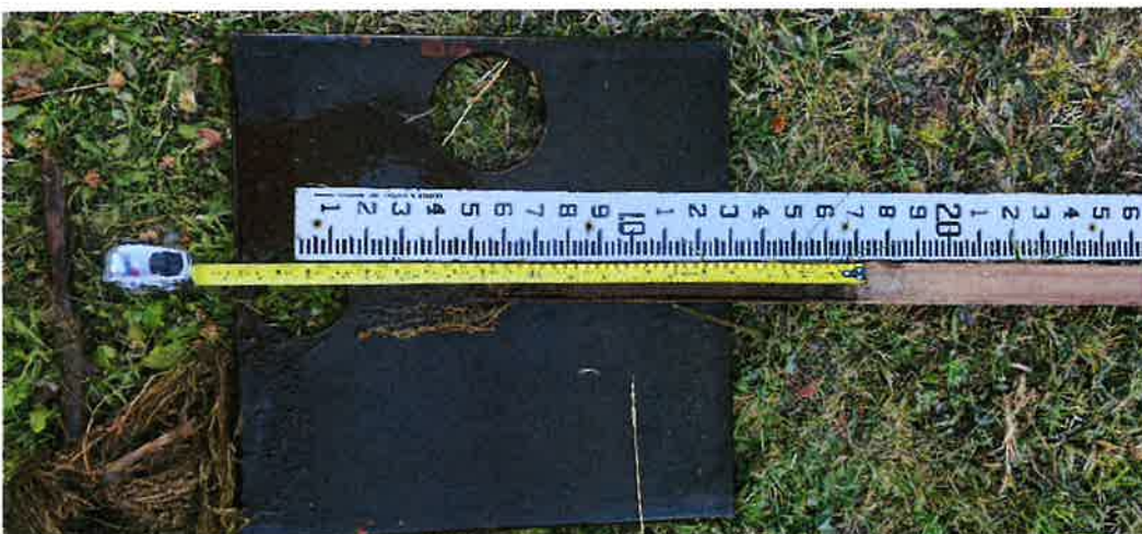
Figure 3: Measuring 3" Orifice to High Water Mark (plate rotates, either orifice can be used)
