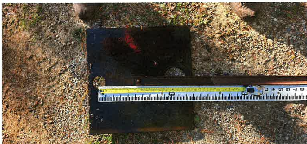
Figure 2: Measurement of 1.5" Orifice on rotating plate. Used 4" orifice for licensing measurement
