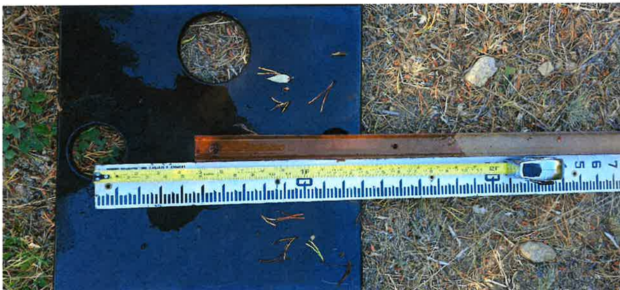
Figure 2: Measuring 3" orifice to High Water Mark on rotating slide plate (used 4" orifice for exam measurement)
