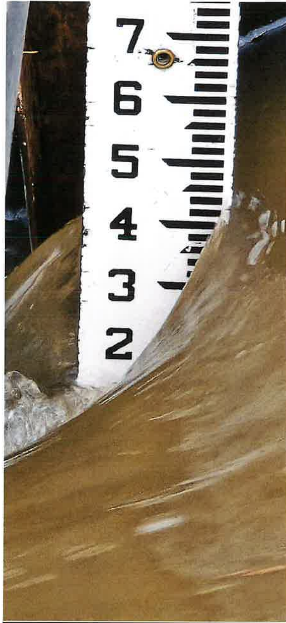
Figure 1: Staff Gauge Measurement at weir of 1.43'
