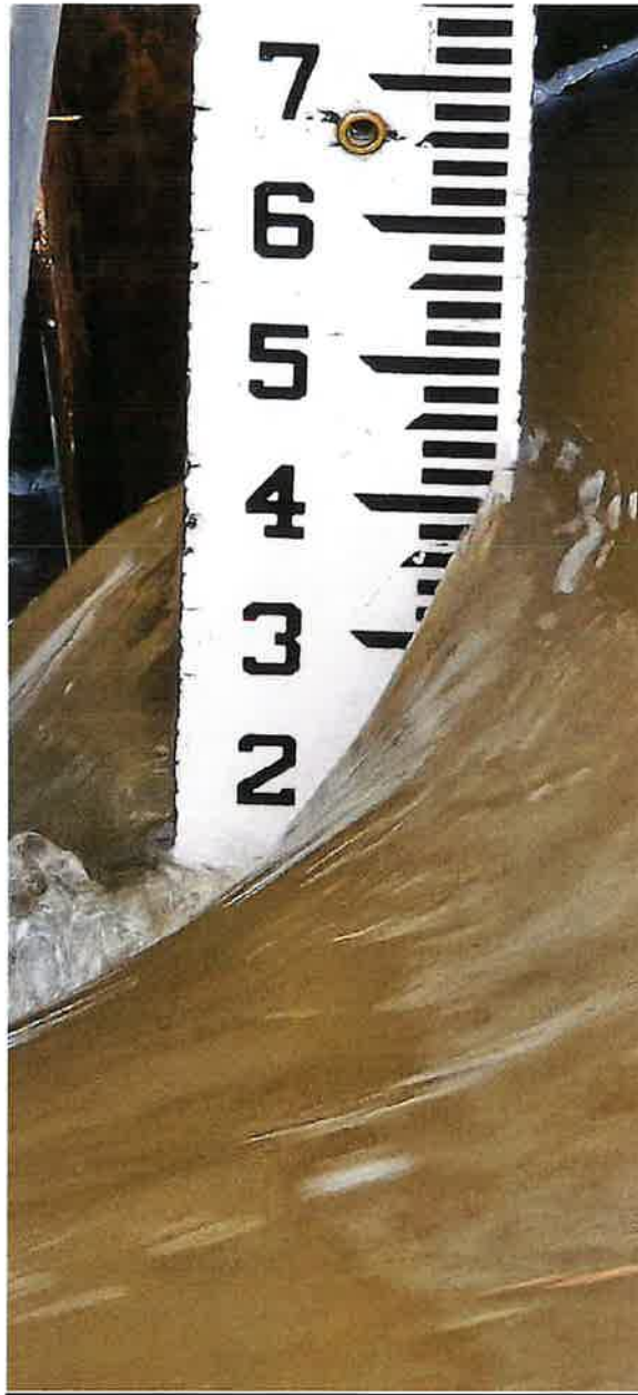
Figure 1: Staff Gauge Measurement at weir of 1.43'
