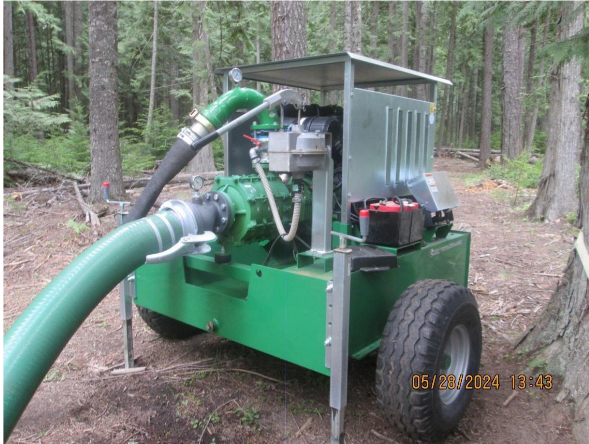
Image 3: 56 HP diesel-powered pump:
