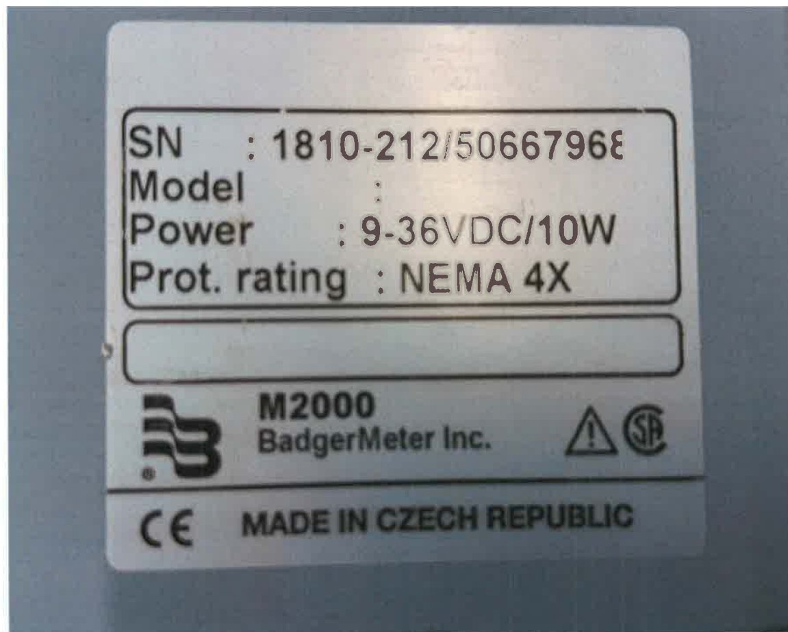
Fig. 6 – Specs for measuring device installed on central line from both wells.
