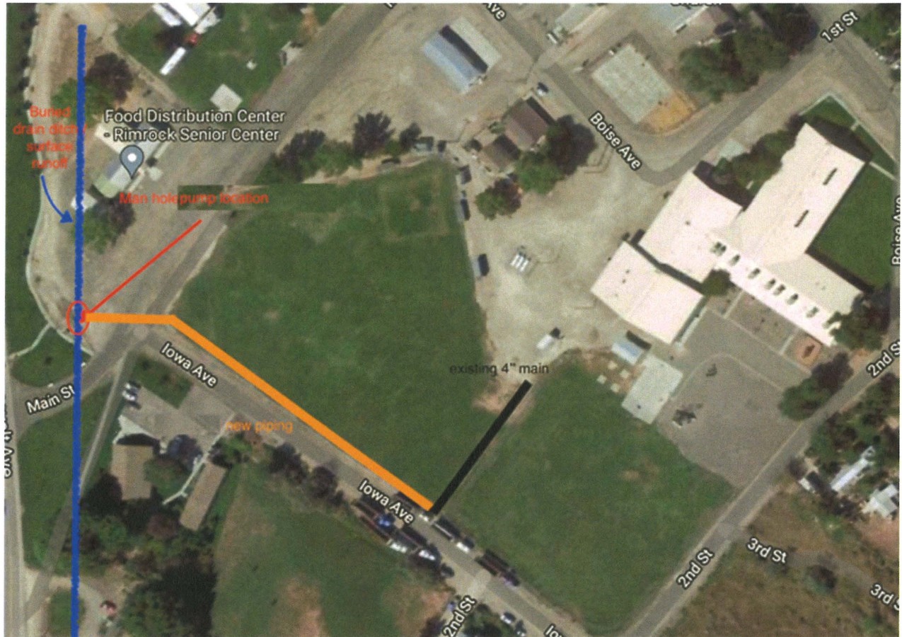
Figure 2 Aerial image provided by permit holder to represent the Snake River drainage ditch including the point of diversion location, labeled "manhole pump location". The orange line represents a water pipe which delivers water to a 4" main pipe between the two main fields, which is then distributed to the sprinklers throughout both fields.
