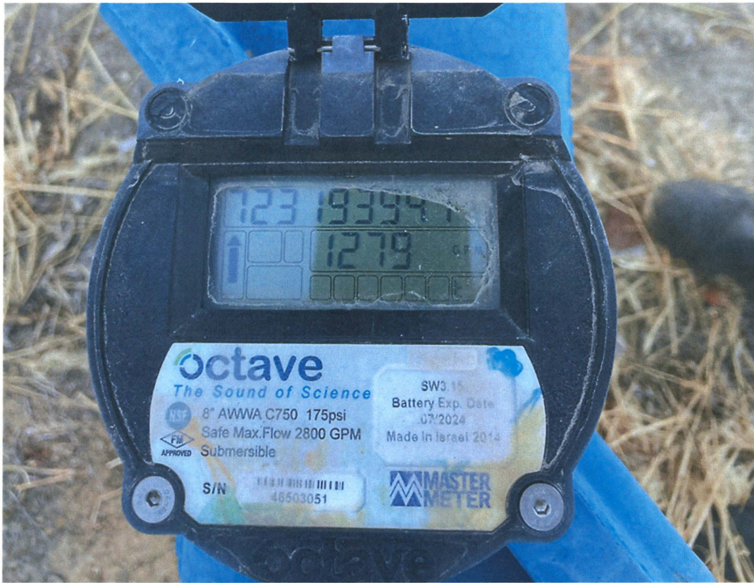
Figure 6 Octave agriculture flow meter reading 1279 gpm at time of field examination.
