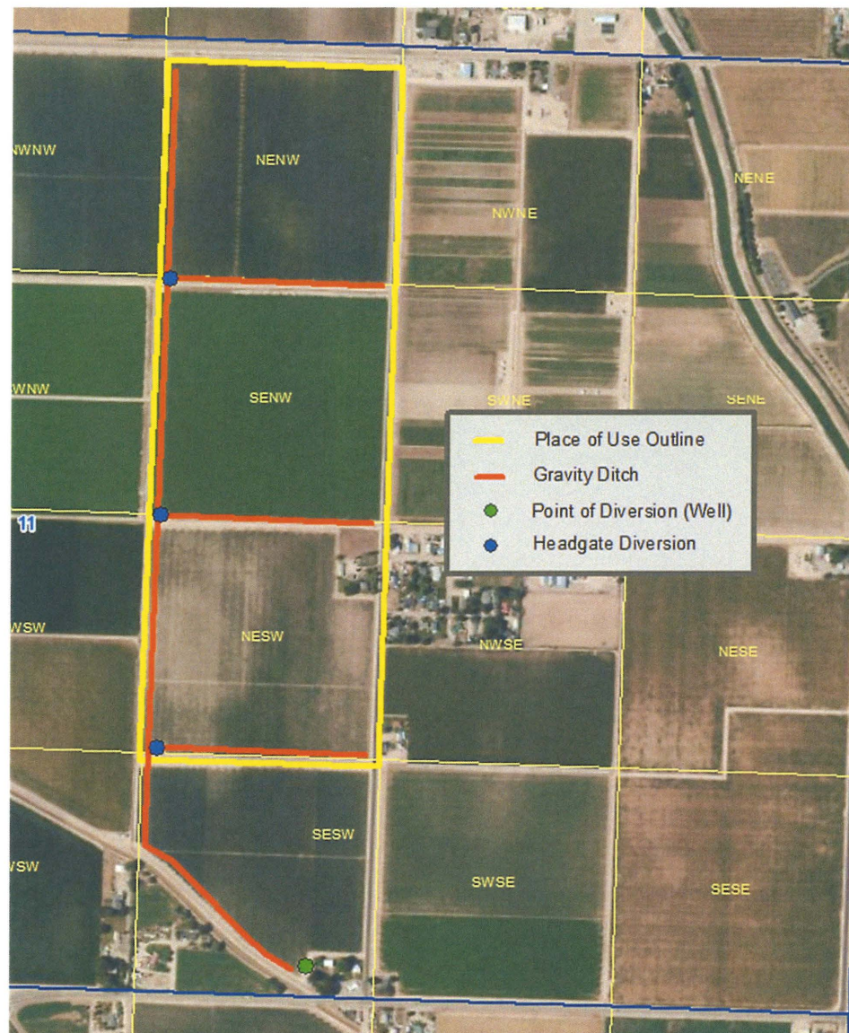
Figure 1 System diagram outlining the place of use, point of diversion location, and irrigation ditch location. The farm is irrigated with a gravity irrigation system including the main ditch, represented with red, and siphon tubes which are placed seasonally and not represented in the diagram.
