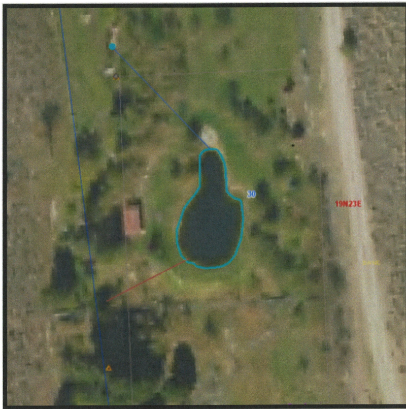
Figure 1- 2023-GIS- imagery of the permit POU (outlined in blue) and POD (blue point). The blue line is the 3" PVC intake from the creek to the north end of the pond. The red line is the 4" PVC overflow drain from the pond returning to Mc Devitt Creek.
