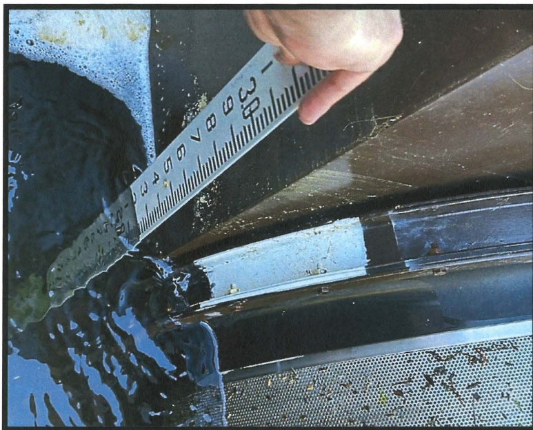
Photo 3- Staff gauge measurement adjacent to the orifice approximately 2.2 ft with highwater mark at 3.1 ft.
