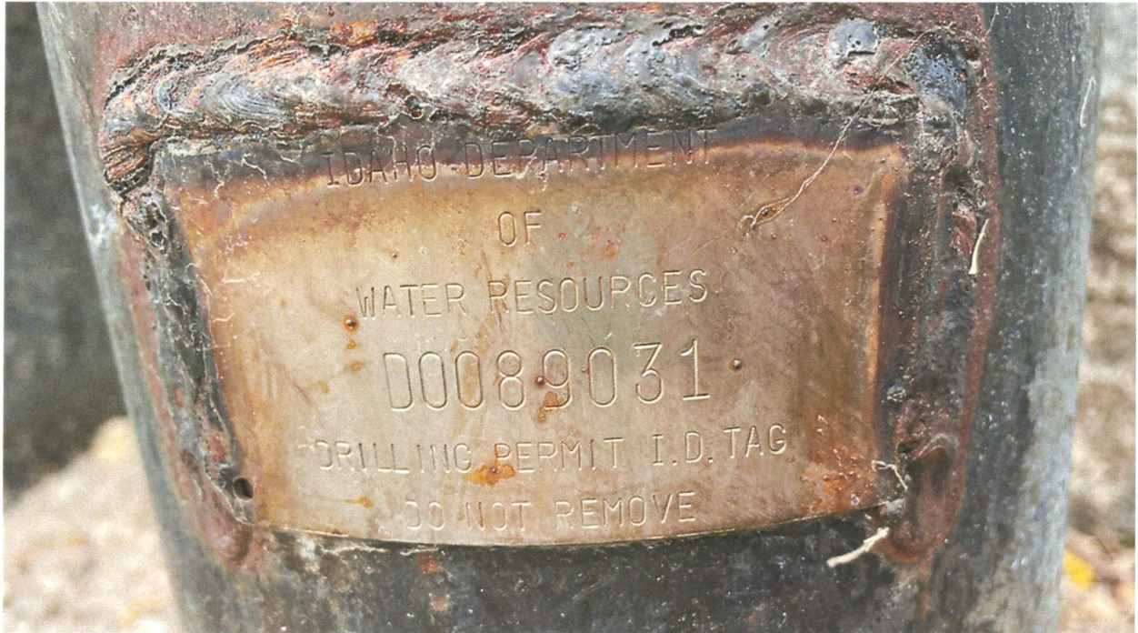
Figure 3 Idaho Department of Water Resources well drilling permit identification tag including the well identification number.
