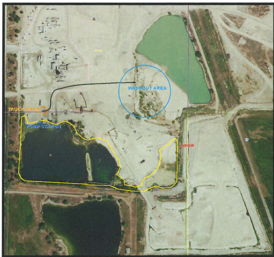
Figures 1a & 1b — System Diagram- 1a. GIS 2017 NAIP Imagery (above) 1b. GIS 2021 NAIP Imagery (below) -Water is diverted via a pontoon pump station with a 25Hp pump that discharges to the elevated filling area.
