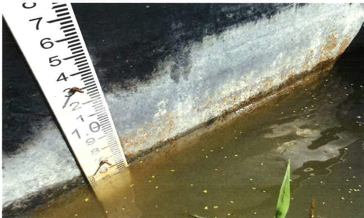
Above: Measuring device from the Dixie Slough, fully contracted standard submerged rectangular orifice with an area of 1.0 ft 2 Water then flows into the delivery ditch to the standpipe.
