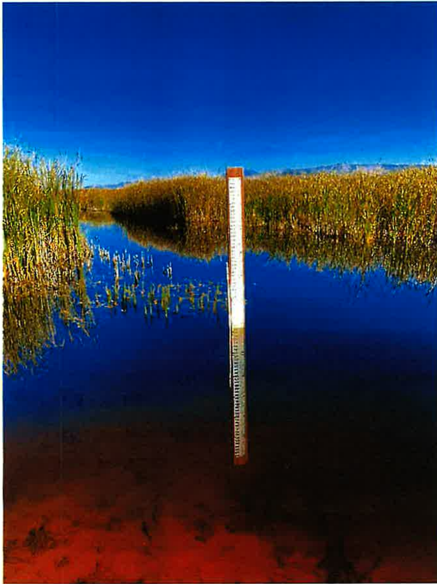
Photo 4. Staff gage in pool adjacent to the eastern point of diversion. A water level logger deployed in the small pipe mounted to the 2x6 wooden board records the water surface elevation of the water stored in Oxford Slough behind the dam.
