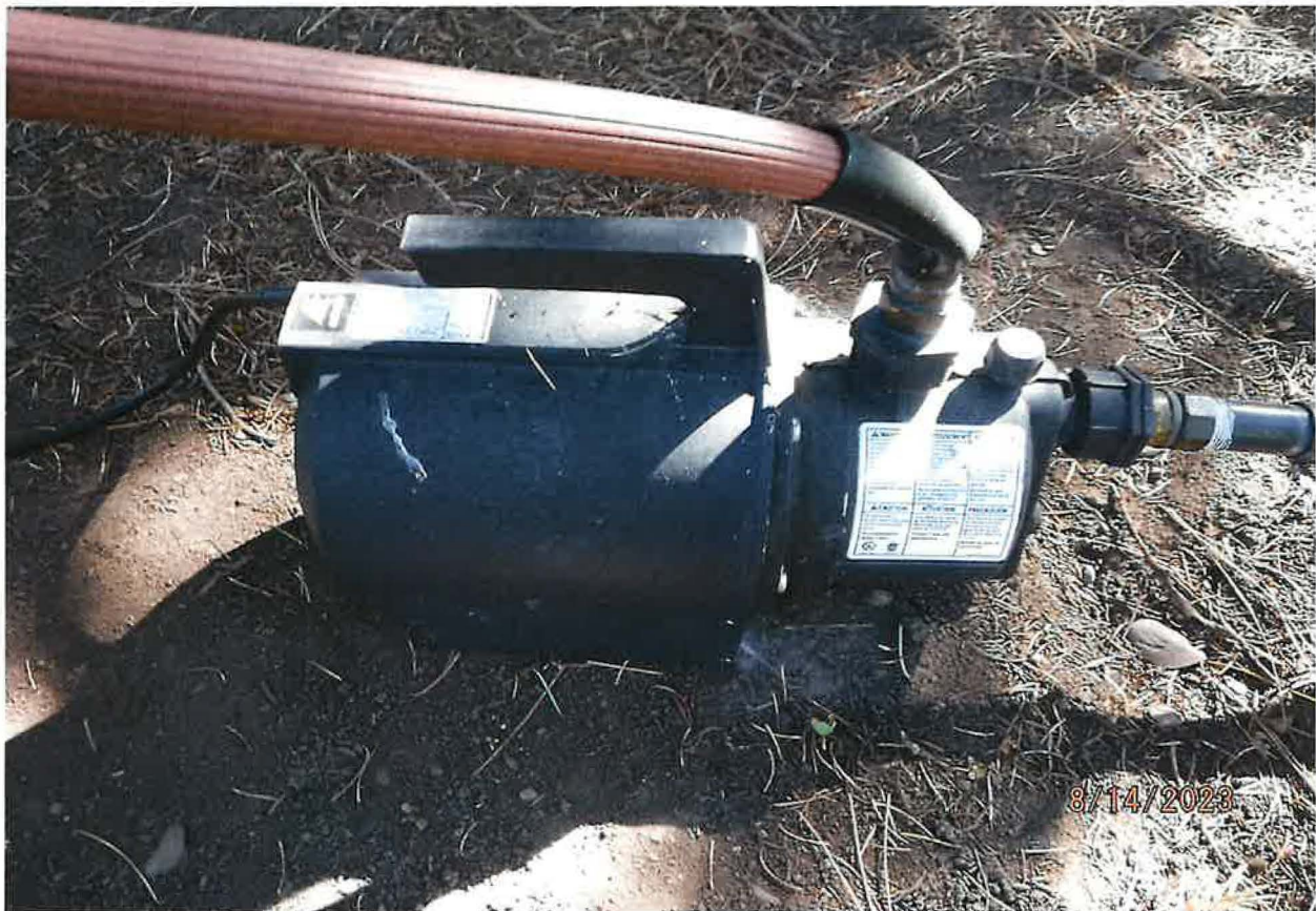
POD – CRAFTSMAN ½ HP PUMP WITH 5/8" HOSE DISCHARGE
