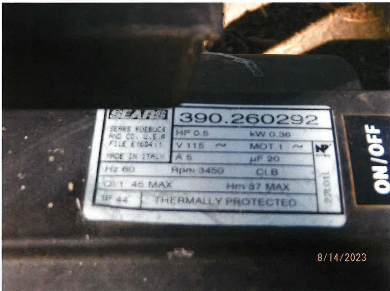
POD – CRAFTSMAN ½ HP PUMP WITH 5/8" HOSE DISCHARGE
