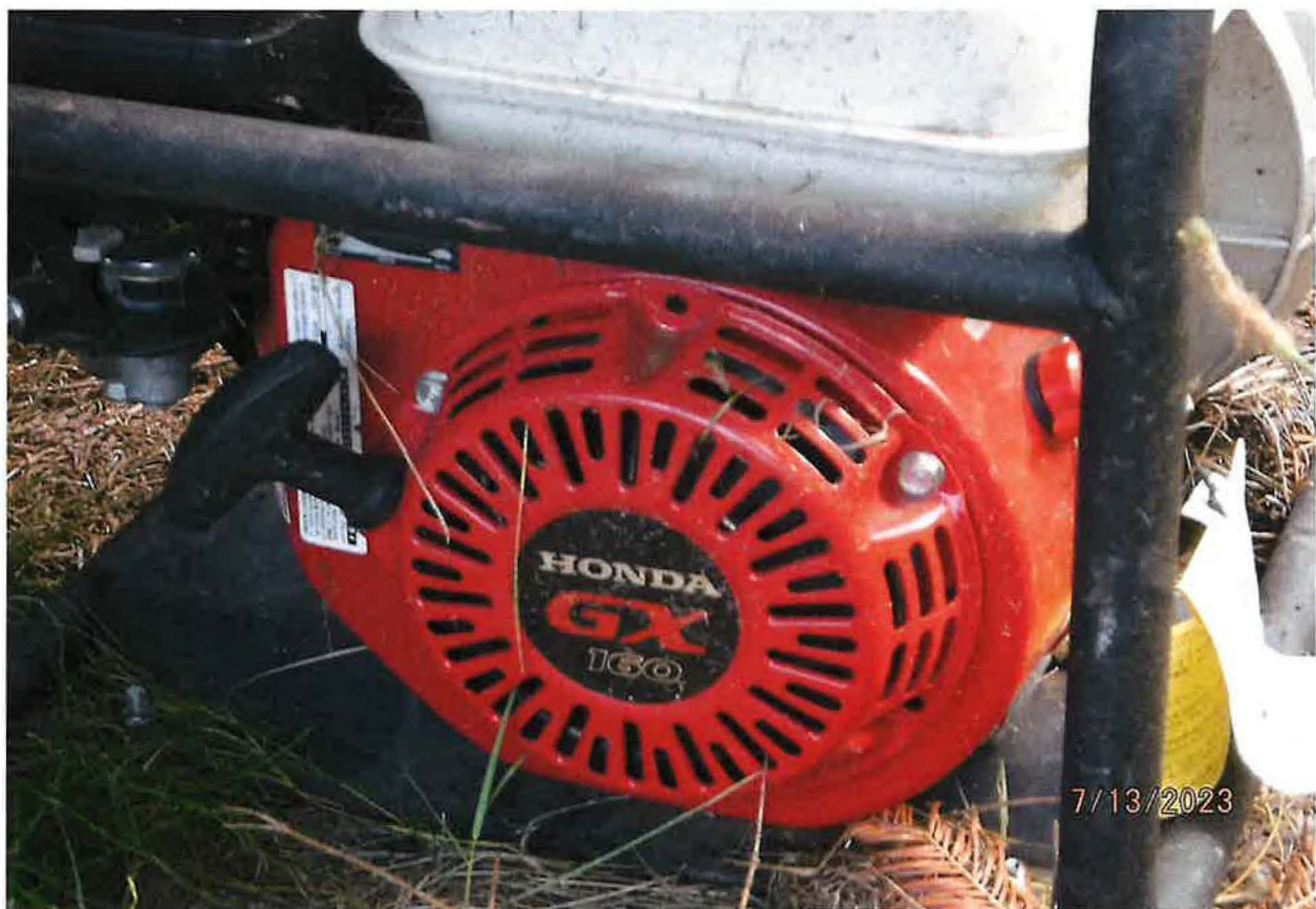
FIRE PROTECTION STORAGE – PORTABLE HONDA TRANSFER PUMP PREPARED FOR USE IN EVENT OF FIRE
