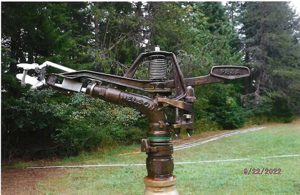
SINGLE NESLON SPRINKLER WITH SINGLE 1 INCH NOZZLE
