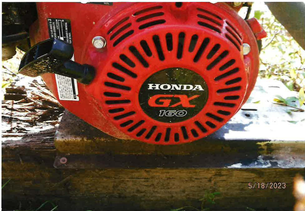
HONDA PUMP AND GX 160 MOTOR WITH 2 INCH INTAKE / 1 ½ INCH DISCHARGE PORT
