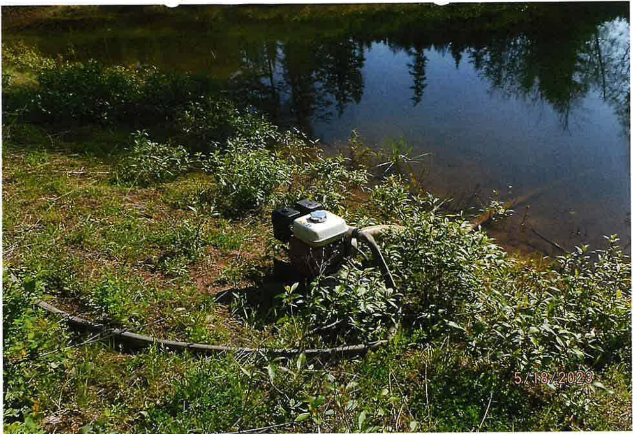
IRRIGATION FROM STORAGE DIVERTING WORKS – HONDA PUMP
