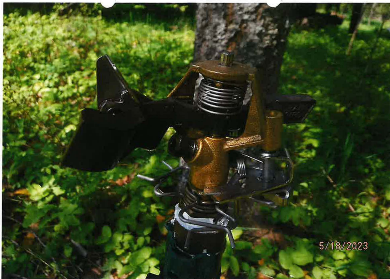
EXAMPLE IMPACT SPRINKLERS USED BY APPLICANT FOR IRRIGATION – 5/32 ND NOZZLE
