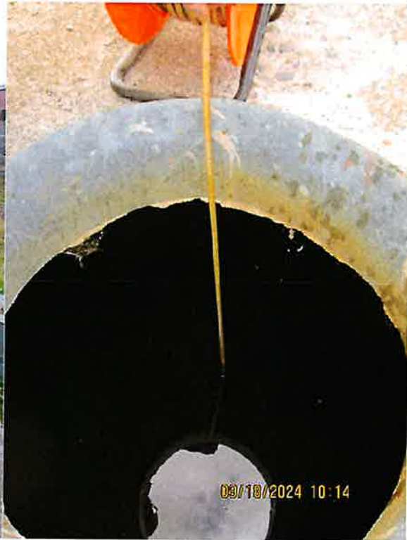
2 & 3) D. Sturgis measuring depth to water in cistern
