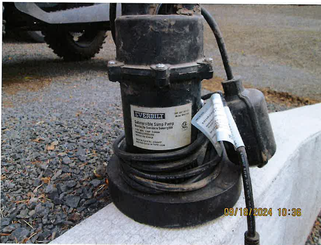
4) Everbilt SBA025BC portable submersible pump used to divert water to stock tanks
