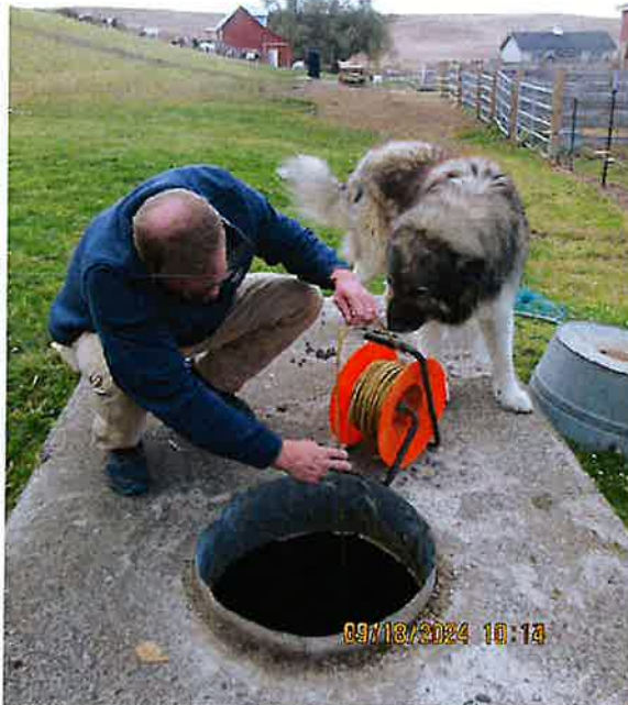
2 & 3) D. Sturgis measuring depth to water in cistern
