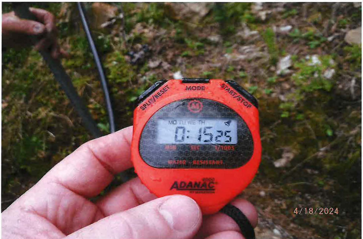
3EA 5-GAL BUCKET FLOW MEASUREMENTS CAPTURED FROM FIRST FROST-FREE HYDRANT INLINE FROM PUMP; LOCATED NEAR RV (FUTURE CABIN SITE)
