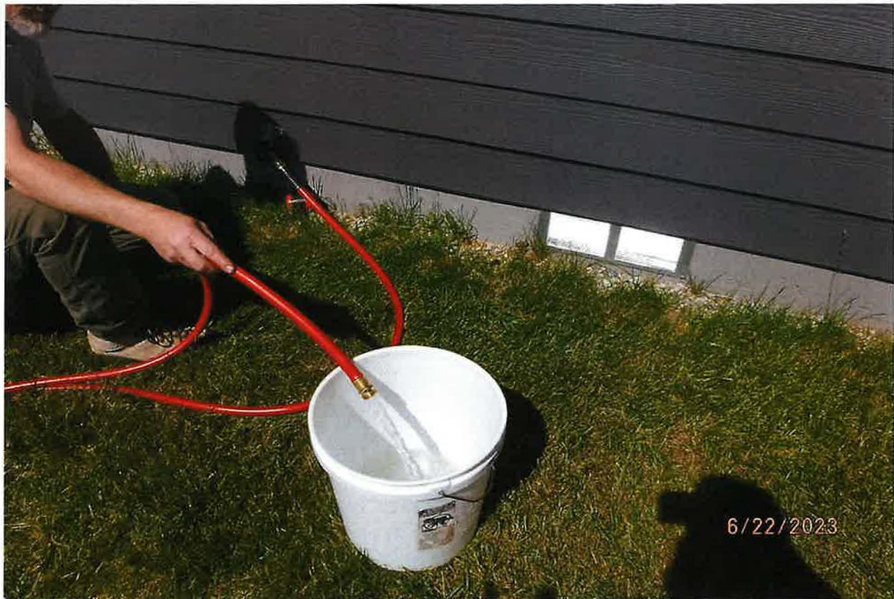
GROUNDWATER FLOW REGULATED TO REDUCE PRESSURE OUTPUT – REDUCES PRESSURE RESULTING IN 6 GPM FLOW RATE FROM HOSE BIB ON SIDE OF RESIDENCE
