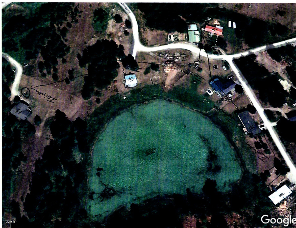
Figure 1- 2023 Google Earth image of Domestic POU emailed to the permit holder who drew a system diagram on it and returned it via email. P=Pump, H= House, and ST= Stockwater tank. A brief description included in the body of the email noted that all pipe was 1" Dia. PVC.
