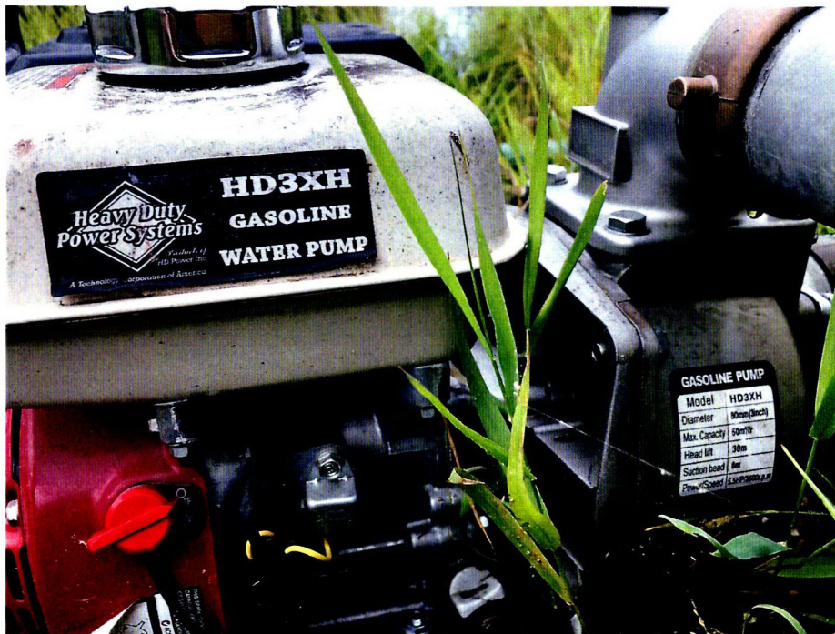
Photo 2- Up close of pump- rated max output+ 60 cubic meters/ Hr.
