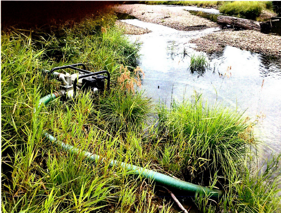
Photo 1- Pump into creek via 4" inlet with fish screen on the intake.
