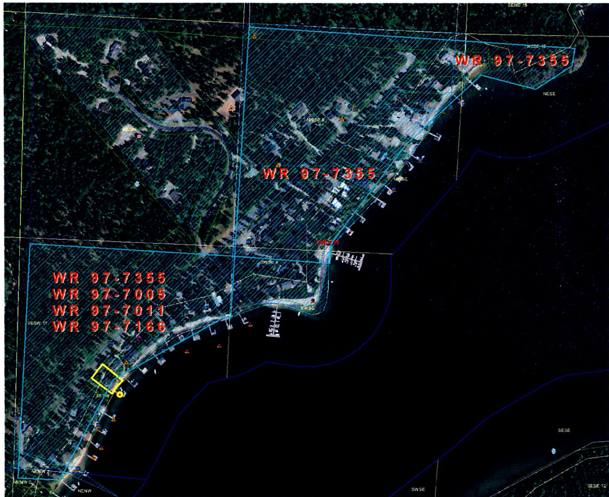
Figure 1.1- Areas outlined in light blue are overlapping water right POU shapes in Arc GIS. Yellow outlined area is WR 97-9586 place of use, yellow point is the respective point of diversion.
