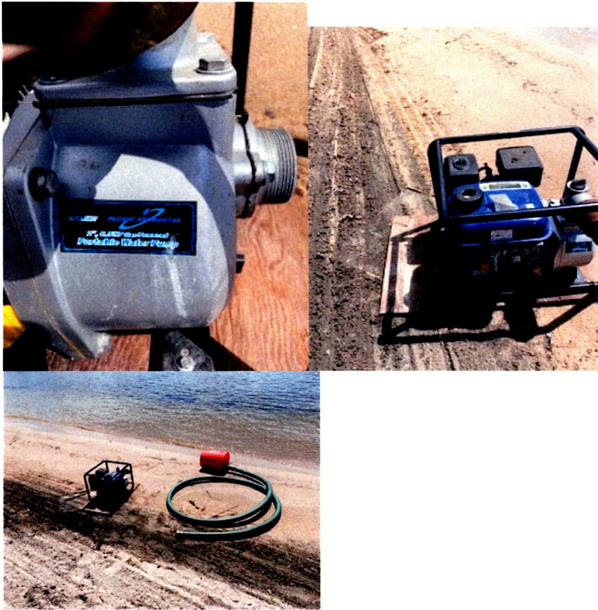
Photos 1, 1.a, &1.b- Images of pump and screened intake. Described in permit holders' email as a 2" diameter, 6.5Hp pump. Pump delivers water to 300 ft of 2" hose to a large portable sprinkler.
