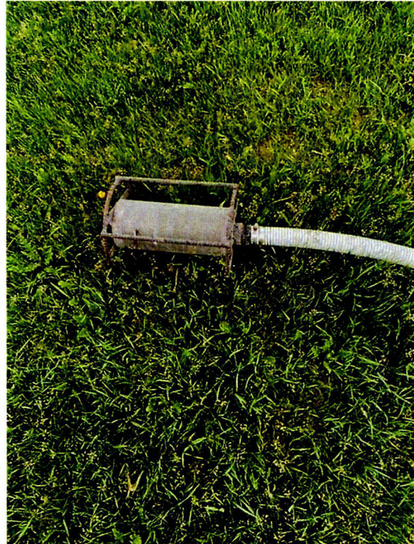
Fish screen on pump intake.
