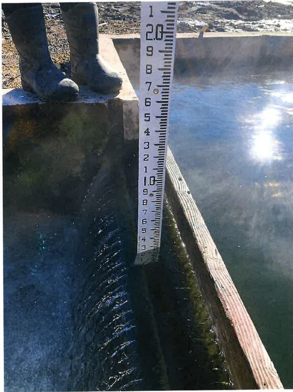
Raceway Rectangular Contracted Weir @ 2.8 inches
