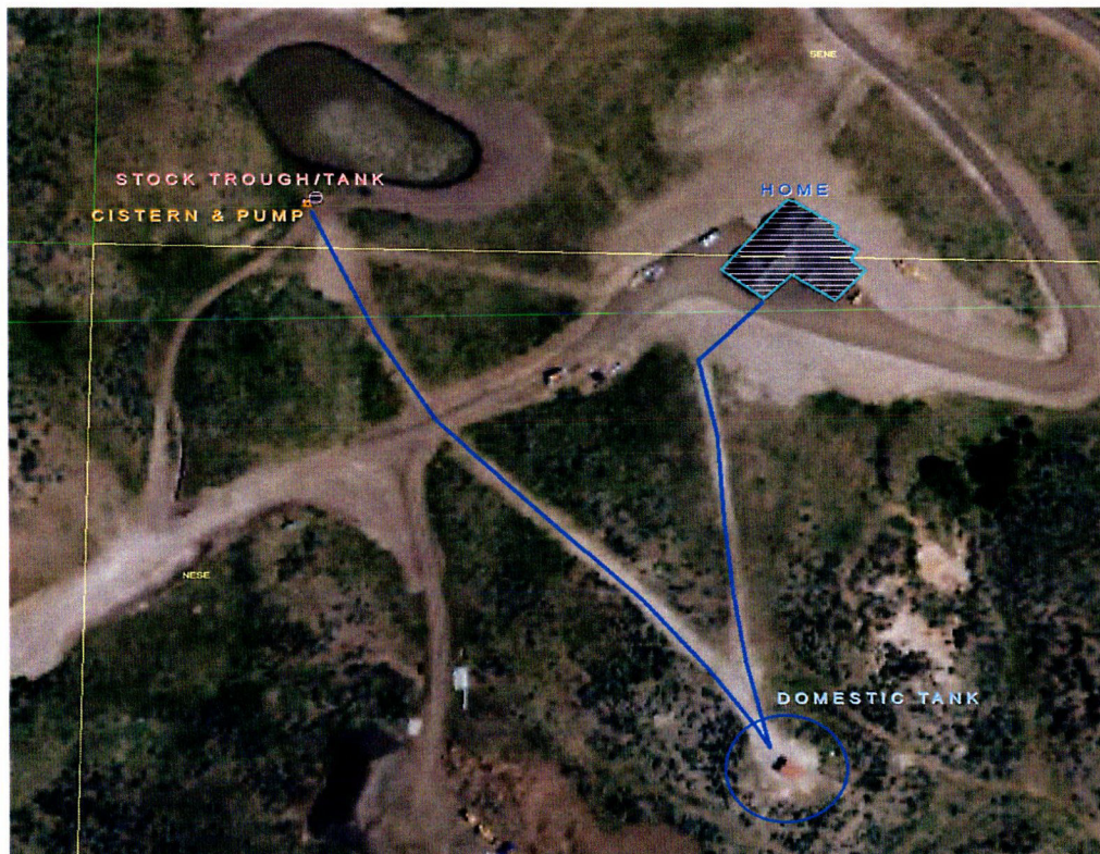
Figure 1.- 2021-GIS image of the system, trench for buried lines evident.
