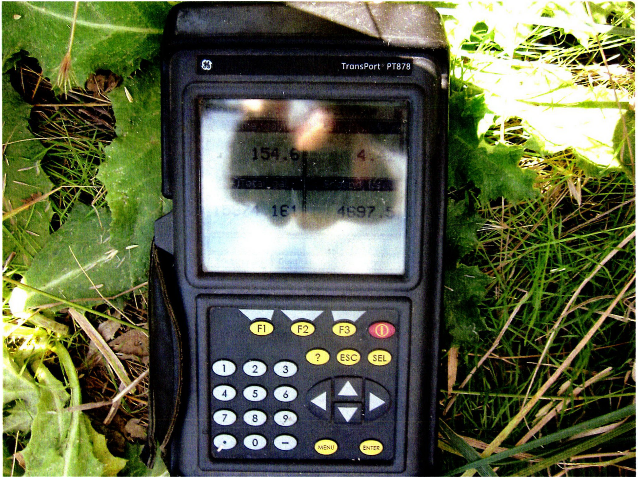
Polysonic Flow Meter: Instantaneous measurement of 154.6 gpm
