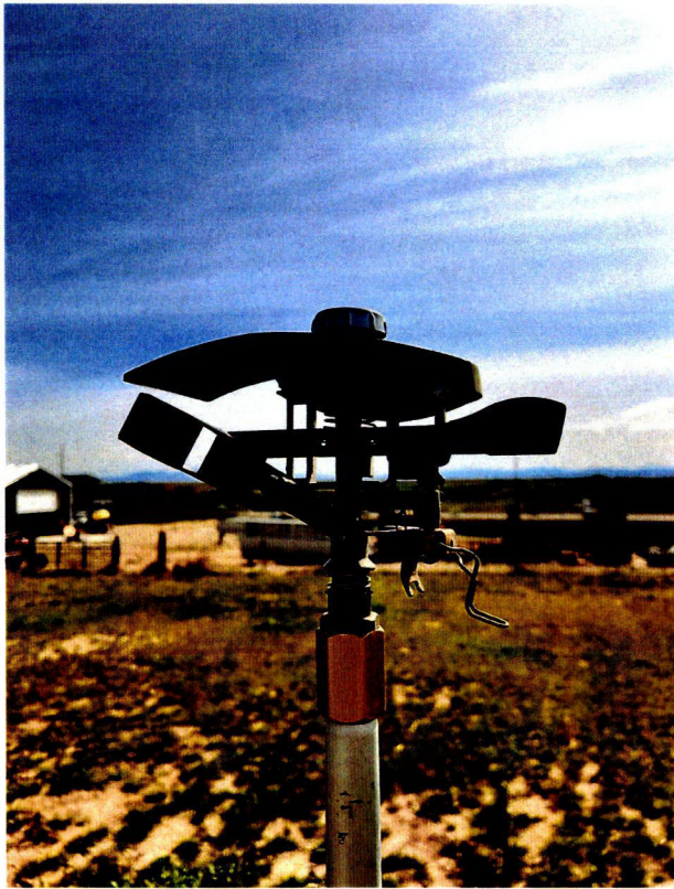
Fig. 11 – Head of sprinkler gun.
