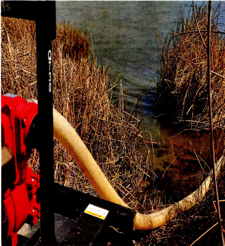
Fig. 3 - Picture of 4" PVC suctions with a 4' ½" lift from the Snake river to pump located in T01N 03W section 8 SWSE QQ. Facing East.
