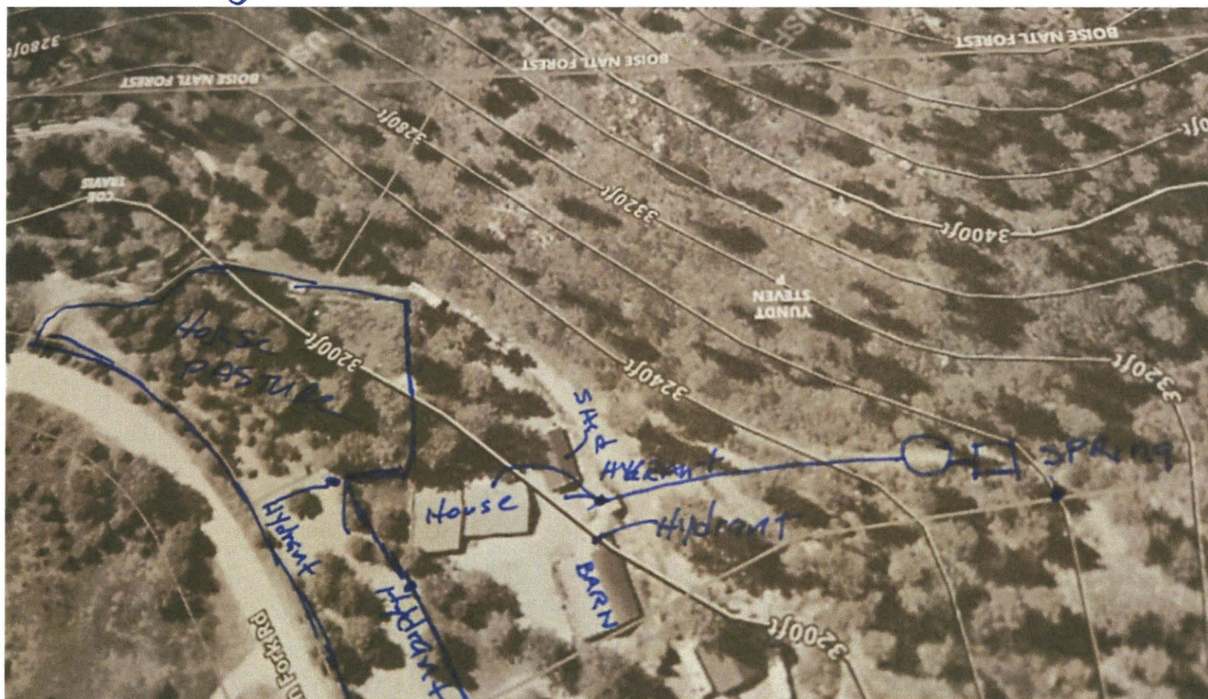
Figure 1 Diagram provided by water permit holder representing point of diversion (dot, labeled "spring"), storage tank represented by a square downhill from spring, irrigated horse pasture, and domestic household
