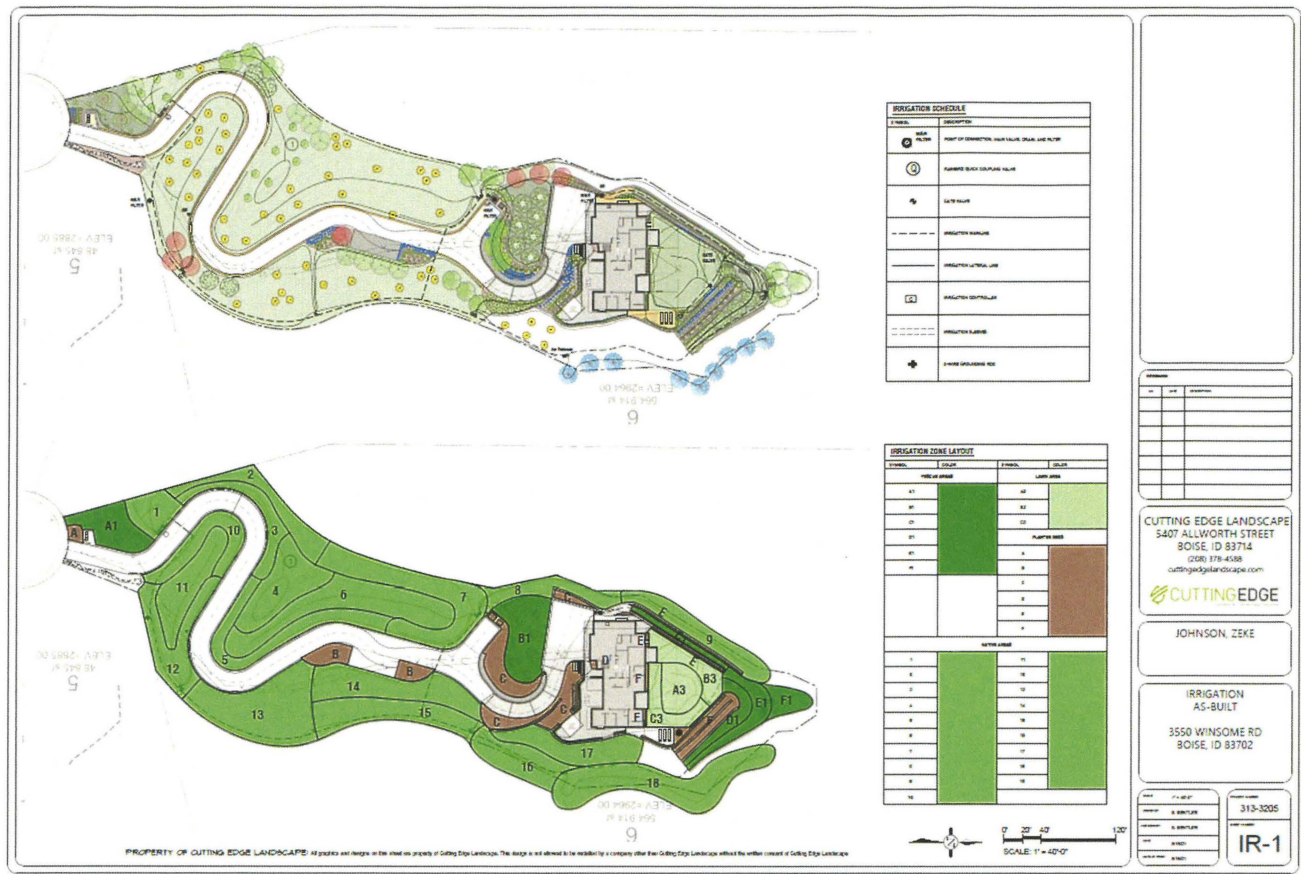
Figure 1 Irrigation as built diagram provided by the owner of this water right. The diagram only represents the owner's personal parcel, totaling to 1.66 acres of irrigated area.
