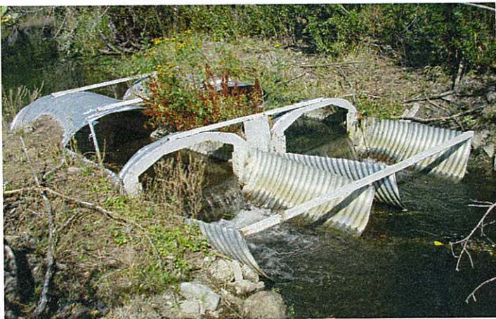
LEFT: View on 9/6/2007 of the measuring device on the Muldoon Ranch Co upper diversion ditch. The measuring device consists of 42-inch rectangular weirs placed in parallel. When the picture was taken, the head through the device was 0.30 feet, which would correspond to about 3.78 cfs of flow.
