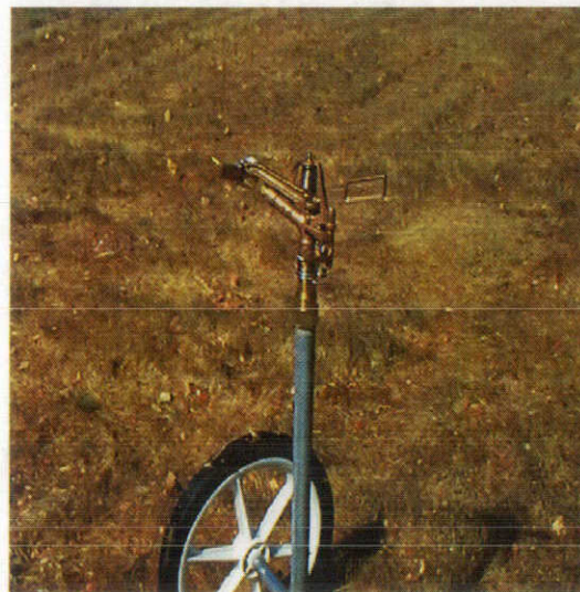
Nelson Sprinkler head, 24gpm
