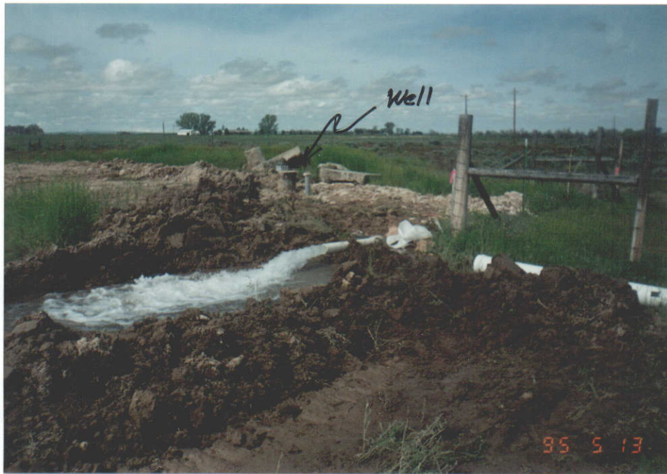
Figure 1 Stutzman 47-08019 Well and 4 inch Pipe Discharging into Ditch
