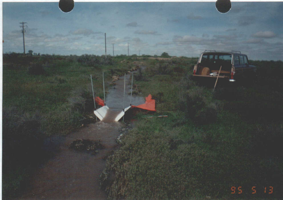
Figure 3 Stutzman 47-08019 Water Measurement with 45° Flume
