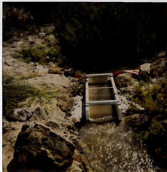
Measuring Weir (Looking Upstream)
