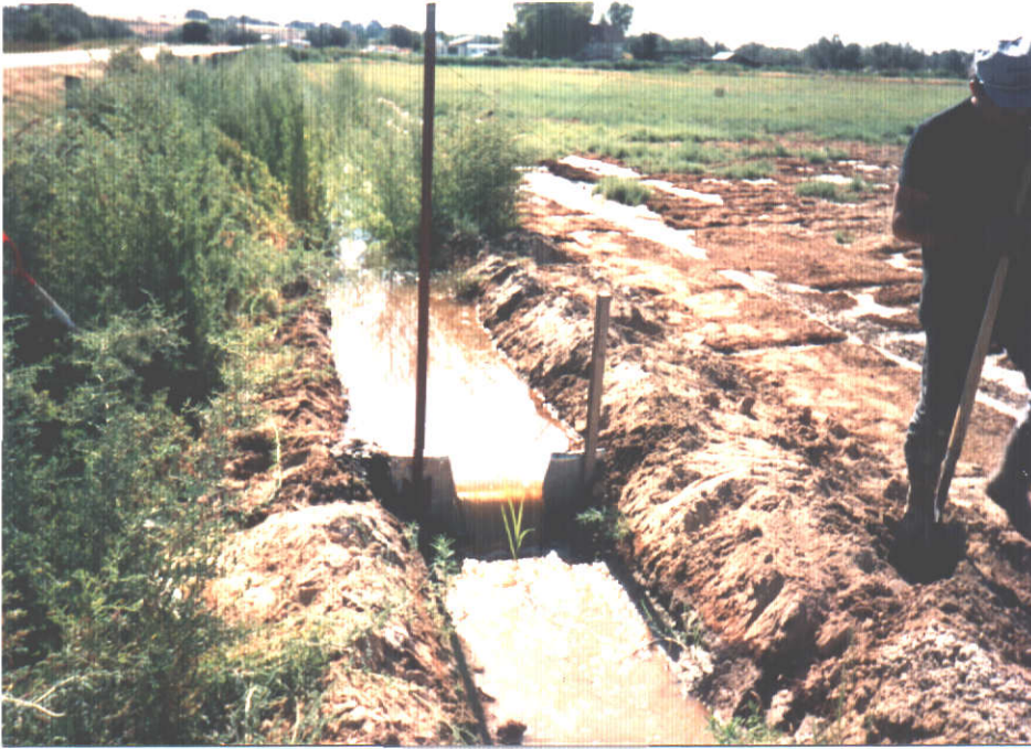
#5 Weir and flow prior to measure- ments of flow.
