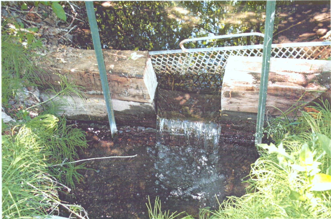
Measuring Point w/Weir Plate Removed By J E Stanton 6-11-2003 Permit 37-8896
