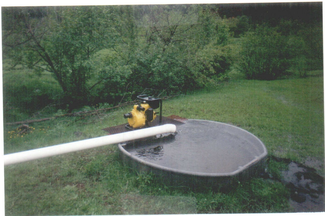
PHOTO ONE- Lockable Device (gate) attached to CMP under ROAD. TOTAL STREAM FLOW is diverted through 4" PVC to STOCK TROUGH.
