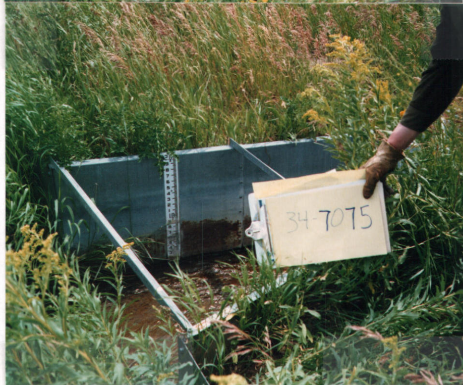
REDIVERSION #1 Parshall flume
