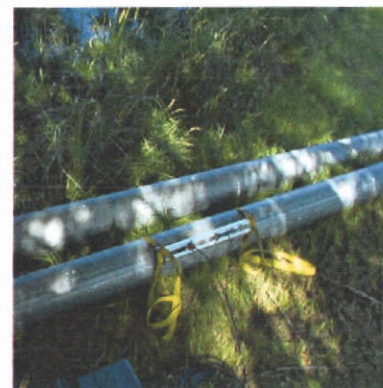
6" aluminum main line and Fuji
