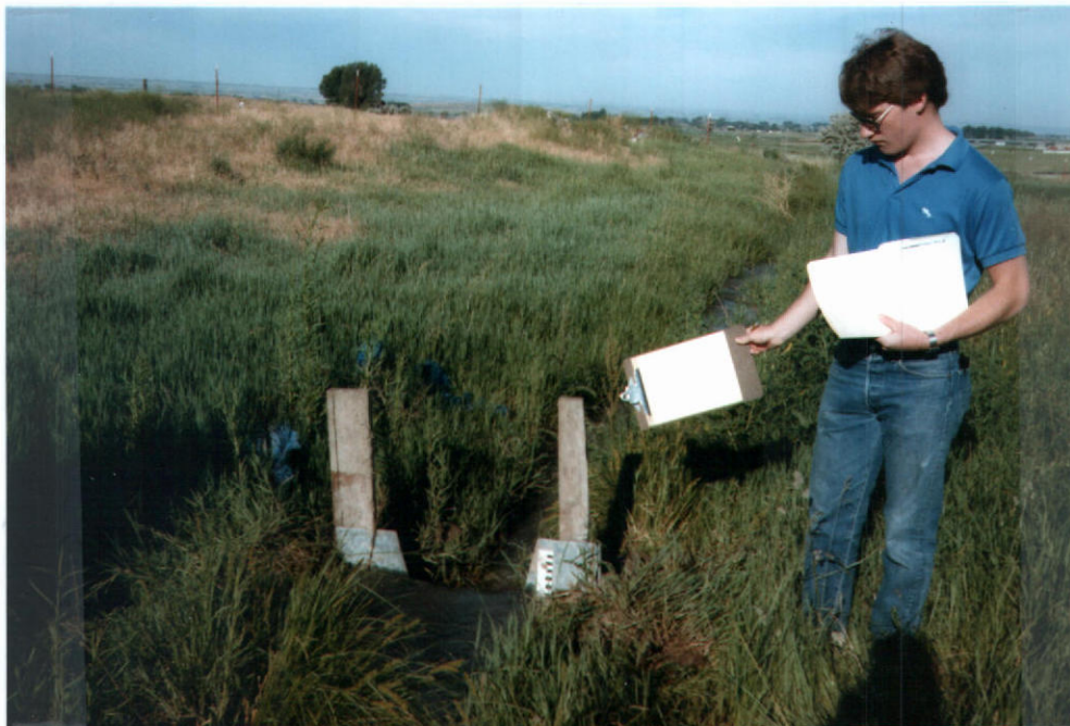
Measuring device is a 1' Cipolletti weir.
