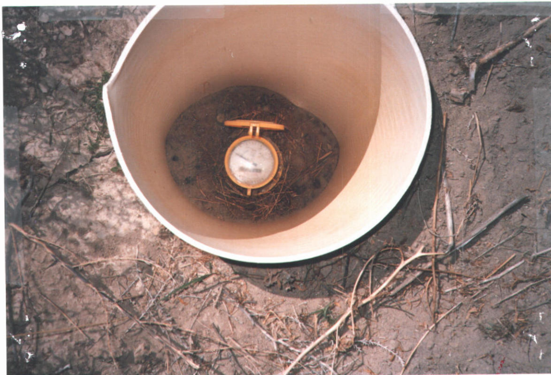
Flow meter reading 500gpm
