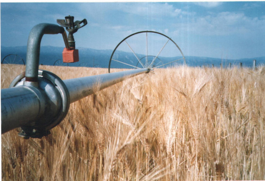
④ Plu, typical sprinkler head on wheel line.
