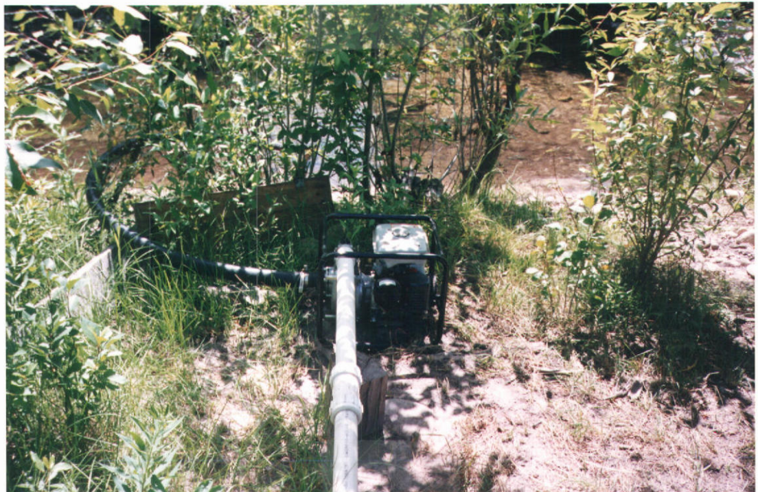
PHOTO TWO- Gas operated 2.7 h.p. pump near Anderson Creek.
